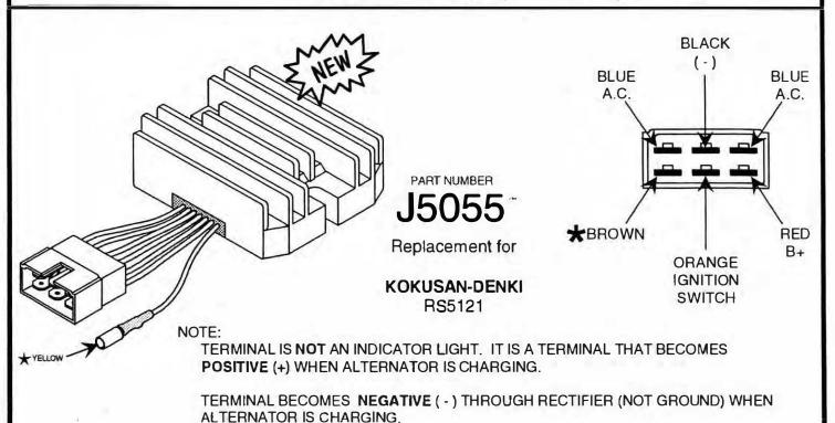
Used on compact tractors and industrial equipment with permanent magnet alternators. Regulator has 7th. wire.
